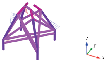
Fig. 7 Horizontal displacement of the upper jacket under extreme load conditions
