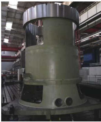
图4 核主泵电机支座(倒置) Fig. 4 Motor pedestal of RCP (upside down)
